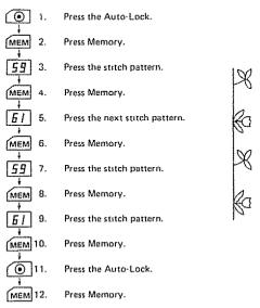
To repeat the same combination of stitches, just press the foot control again after stitching the first combination.
